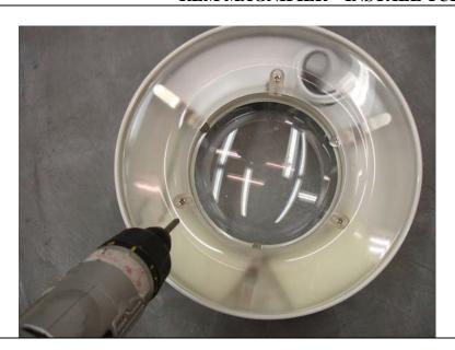
REMOVE 3 SCREWS WITH PHILLIPS SCREWDRIVER
