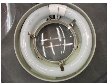
PLACE TUBE IN HOUSING AND SECURE WITH 3 RETAINERS
